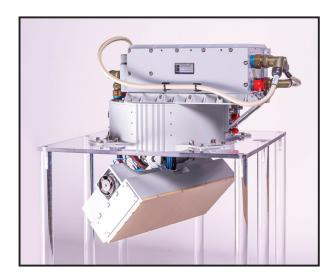
The Guardian generates high-resolution SAR images for the detection and visualization of detailed features of the scenario, enabling classification of various targets in all weather conditions and during day and night.
