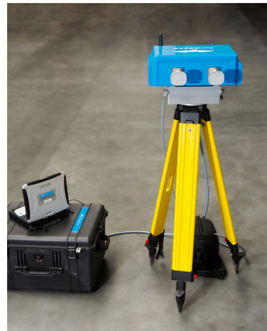
FastGBSAR-R installed on a tripod
