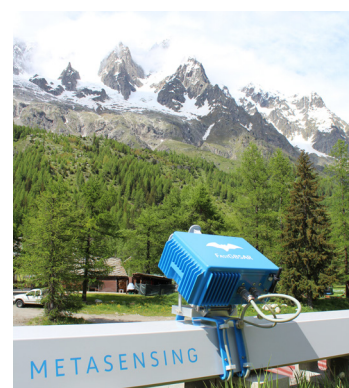
Figure 4. View of the FastGBSAR-S installed in front of the glacier in the Italian Alps.
