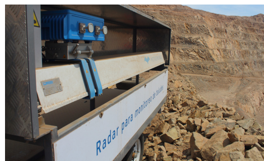
Figure 5. View of the FastGBSAR-S in an open pit mine.
