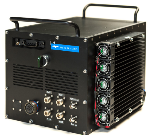
The MetaSAR-X enclosure is compact and light-weight, allowing for quick and flexible mounting.
