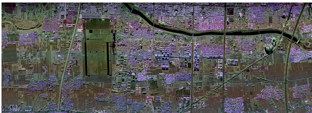
Color-coded composition of fully polarimetric X-band intensity images acquired over a urban scenario. The SAR image has a ground range of 3.5 km and an azimuth range of 10 km. (Red: VV, Green: HH, Blue: VH).
