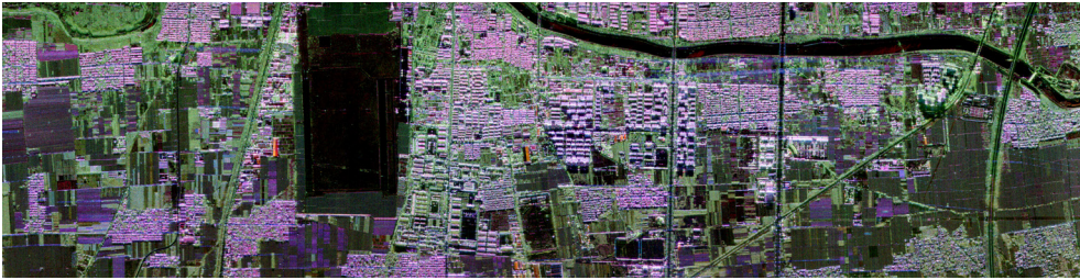
Color-coded composition of fully polarimetric L-band intensity images acquired with the MetaSAR-XL. (Red: VV, Green: HH, Blue: VH)
