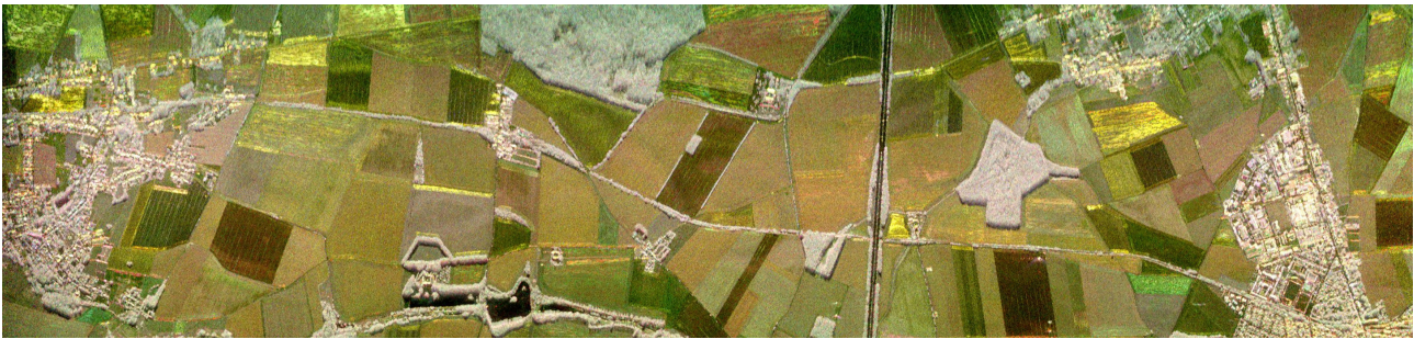
Polarimetric airborne bistatic SAR image obtained with two independent MetaSAR-L on two aircraft flying in formation. Red, green and blue correspond to HH, VV and HV pol channels.
