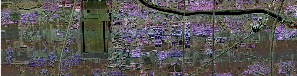
Color-coded composition of fully polarimetric X-band intensity images acquired with the MetaSAR-XL. (Red: VV, Green: HH, Blue: VH)
